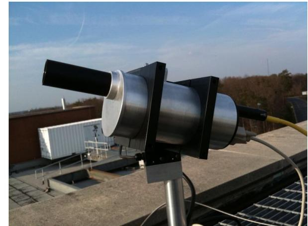
**(Left)** Pandora head sensor on dedicated stand. **(Right)** Head sensor contains up to two filter wheels for polarizers and filters. Internal microcontroller controls tracker and Interfaces with data acquisition computer.
